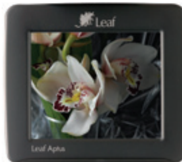
Right: Rear screen on Leaf Aptus 75 digital camera back, showing full screen (6x7cm) view of captured image on the touch screen and (far right) an enlarged view.
